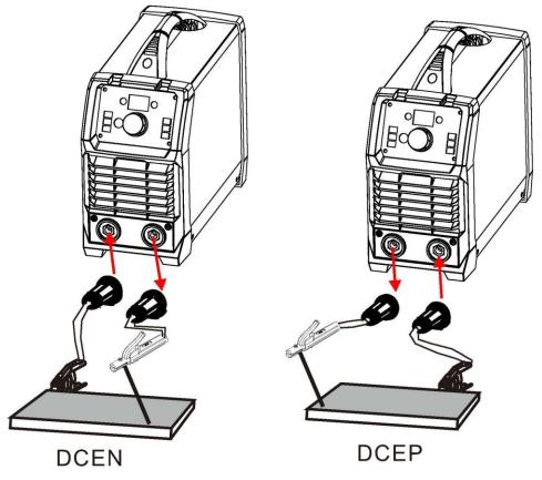
power cable connected to the appropriate position, not to pick the wrong voltage;
