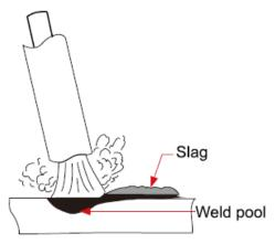
Manual metal arc (stick) electrodes have a solid metal wire core and a flux coating. These electrodes are identified by the wire diameter and by a series of letters and numbers. The letters and numbers identify the metal alloy and the intended use of the electrode.
