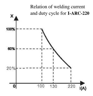
welding current OFF and light the over-heat pilot lamp on the front panel. In that case, the machine should not be welding for 10-15 minutes to cool down with the fanrunning. When operating the machine again, the welding output current or the duty cycle should be reduced.
