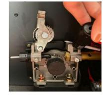
6.At the wirefeed assembly, release the compression screw by swivelling it outwards. This allows the top roller arm to spring to the open position. The end of the welding wire can now be passed through the inlet guide, over the bottom driven roller, and into the output wire guide tube.
