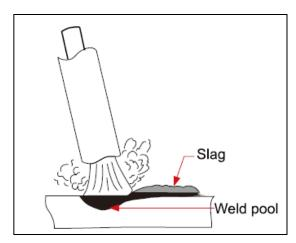
The covering on a shielded metal arc welding electrode is called **Flux**.
