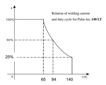
signal to the welding machine control unit to cut the output welding current OFF and light the over-heat pilot lamp on the front panel. In that case, the machine should not be welding for 10-15 minutes to cool down with the fanrunning. When operating the machine again, the welding output current or the duty cycle should be reduced.
