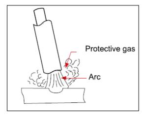
Manual metal arc (stick) electrodes have a solid metal wire core and a flux coating. These electrodes are identified by the wire diameter and by a series of letters and numbers. The letters and numbers identify the metal alloy and the intended use of the electrode.
