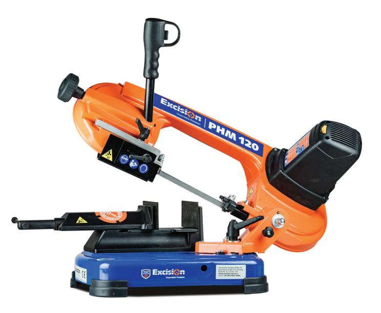
The PHM120 is a compact and portable bandsaw, boasting a generous 120mm capacity. Its variable speed motor offers an impressive range of 30-80m/min, enabling efficient cutting of both tough steels and non-ferrous materials.
