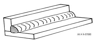
Figure 5-5: Horizontal - Vertical (HV) position
