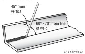
Figure 5-14: Electrode position for HV fillet weld
