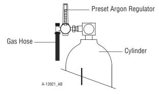
Figure 6-1: Fit Regulator/flowmeter to Cylinder
