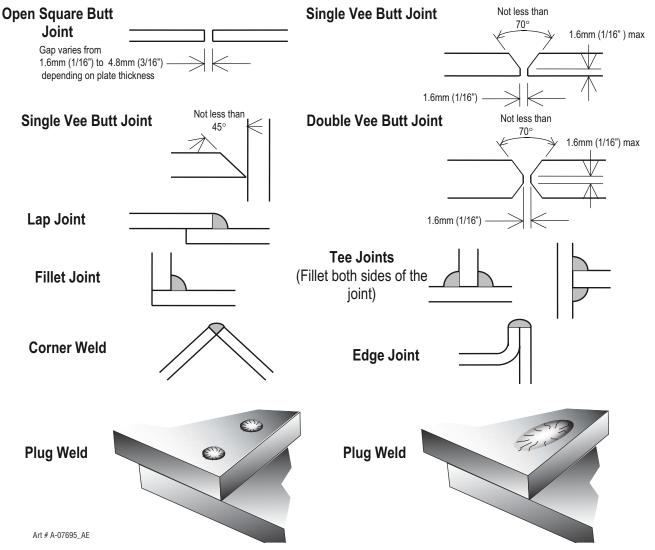
Figure 5-10: Typical joint designs for arc welding
