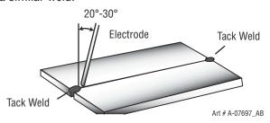
Figure 5-12: Butt weld
