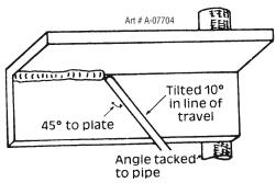
Figure 5-19: Overhead fillet weld
