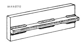
Figure 5-27: Chain intermittent welding
