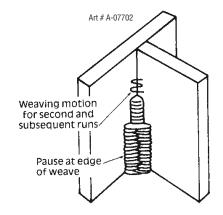
Figure 5-17: Multi run vertical fillet weld
