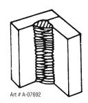
Figure 5-7: Vertical position, fillet weld
