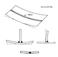
Figure 5-24: Examples of distortion
