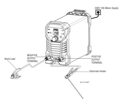
Figure 5-1: Setup for STICK (MMAW) Welding
