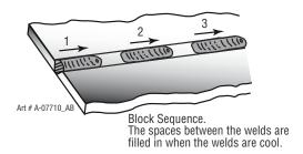
Figure 5-25: Welding sequence
