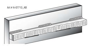
Figure 5-28: Staggered intermittent welding
