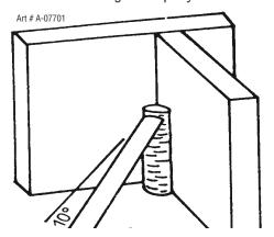
Figure 5-16: Single run vertical fillet weld
