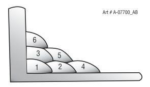
Figure 5-15: Multi-runs in HV fillet weld
