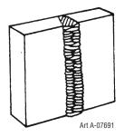
Figure 5-6: Vertical position, butt weld
